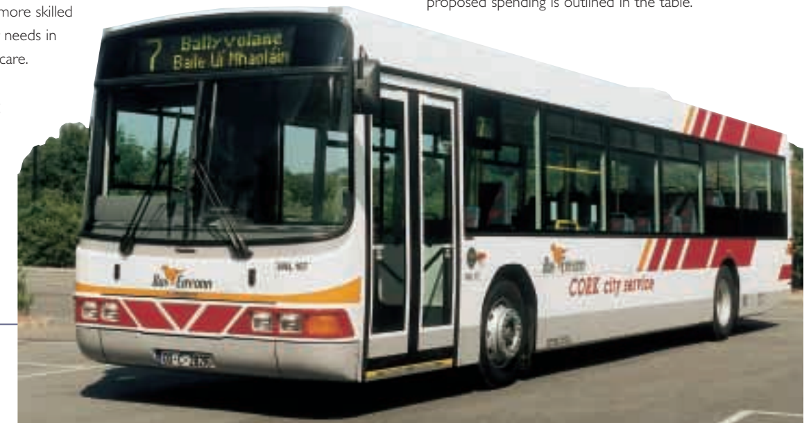
Bus Éireann's first city service buses to be part-funded under the National Development Plan are Volvo Wright low-floor vehicles which can accommodate 45 seated and 27 standing passengers. They also have a wheelchair space and are fully accessible to people who are mobility impaired.
